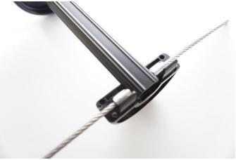
4. Place additional standoff halves on top of standoff halves supporting ladder rung, apply light pressure until the halves snap together. NOTE: It may be necessary to apply tension or a slight twisiting motion to rope ladders to stop the halves from pinching rope during assembly.
